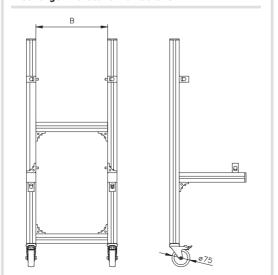
The swivel casters used have a total locking device, which guarantees a secure footing even at high transport speeds. The height and width of the stand is adapted based on the configuration; see the order example on the right.
