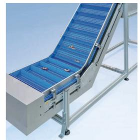
Incline conveyor modular belt KFM-P 2040 with protective box on the infeed end
