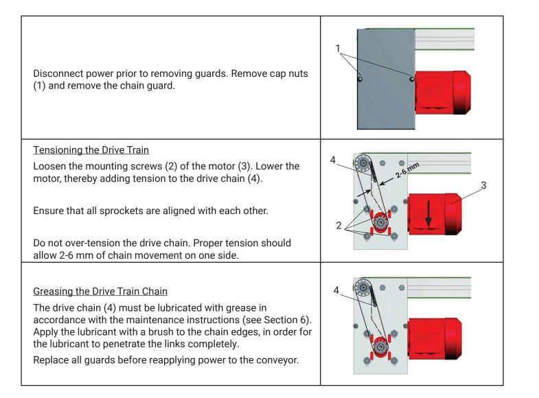
\*Reassemble in reverse order; ensuring all screws are tight and all guards are in place before operating.
