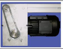
Remove chain guard as described above. Apply luubricant, as called out in Section 6, with a brush to the chain edges in order for the lubricant to penetrate the chain completely.
