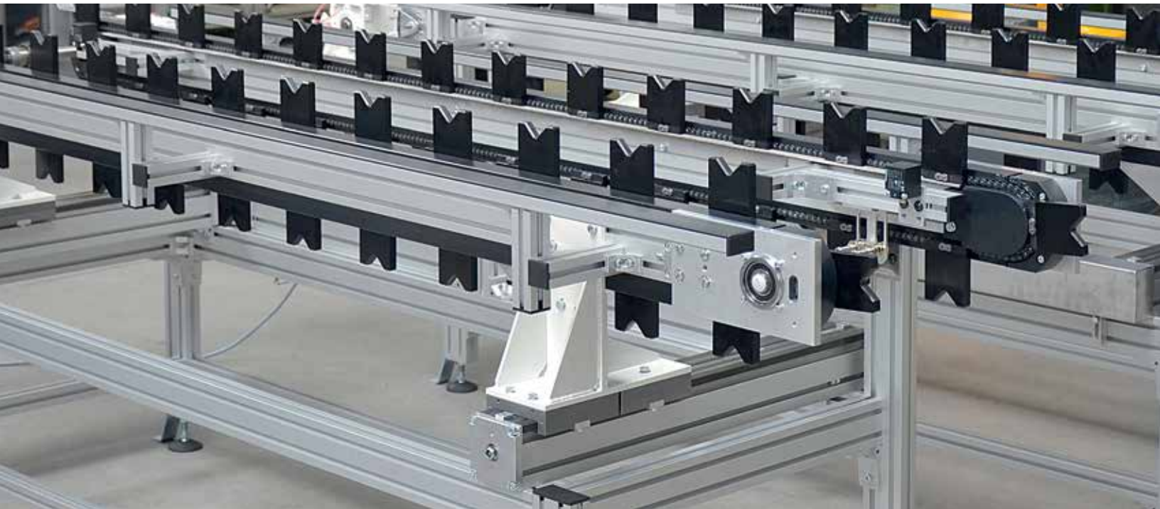
TKU 2040 adjustable width unit. This conveyor also features oversized POM fixtures.
