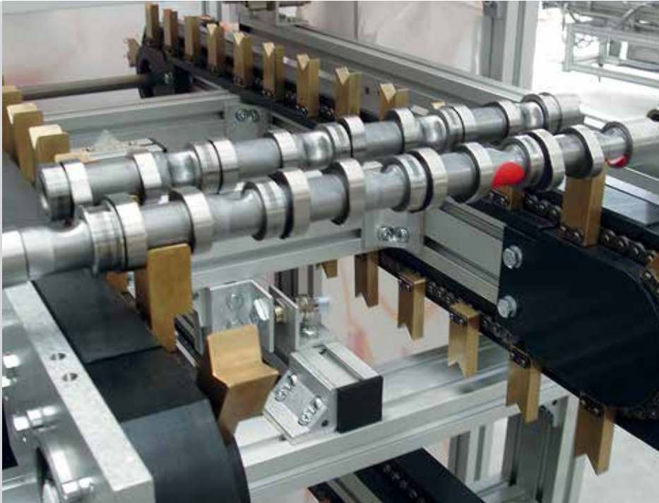
TKU 2040 fixed width conveyor that is also capable of handling parts of various lengths.
