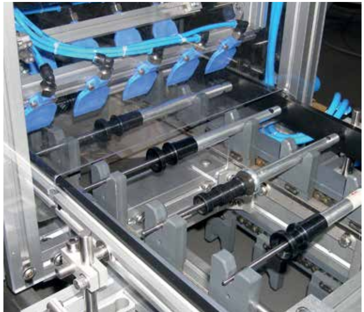
A TKU 2040 conveyor integrated into a custom parts cleaning operation.
