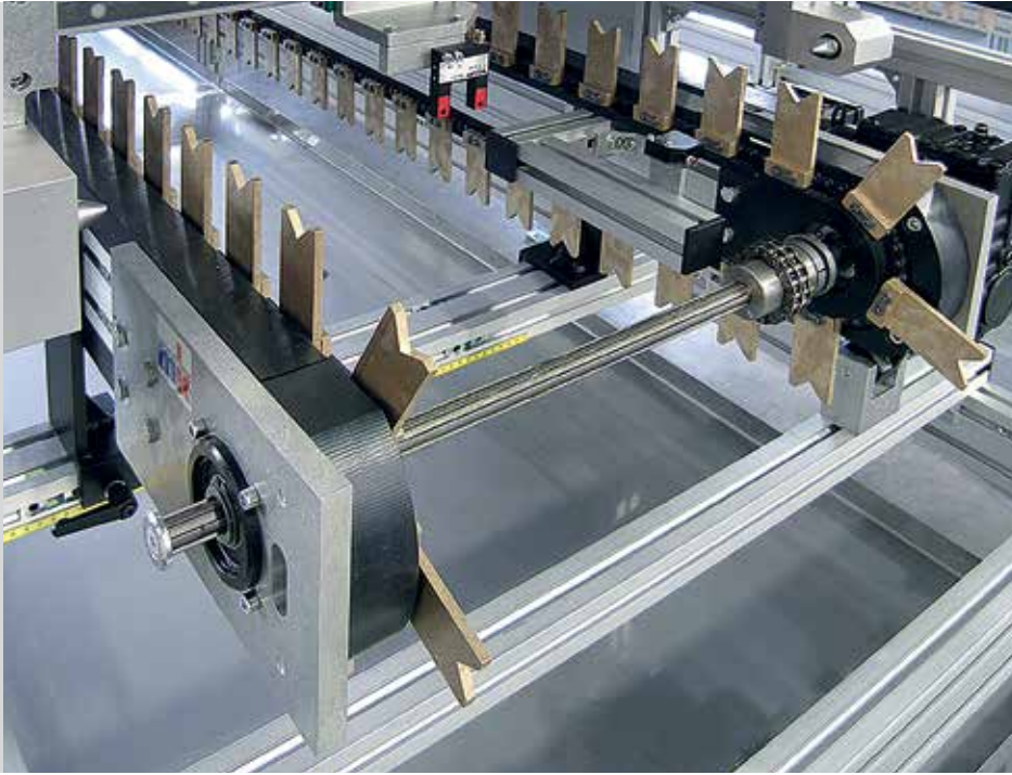
TKU 2040 with manual width adjustment and brass fixtures.
