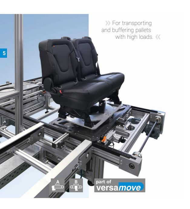
The accumulating roller chain conveyor SRF-P 2010 is particularly suitable for transporting pallets (in the Versamove pallet circulation system, for instance). The free-spinning conveyor rollers run smoothly, even during accumulated operation. They also keep back-pressure forces to a minimum. Typical applications include interlinking or buffering between workstations and building complete transfer lines.
