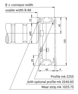
270 Roller Conveyors Roller Conveyors 271
