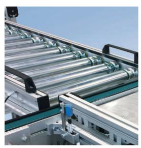
Drive roller conveyor RBM-P 2255 with maintenance access
