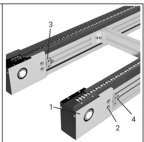
Chain is properly tensioned when the chain can be lifted a max. of 1-2 mm.
