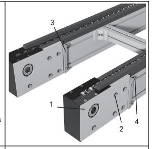
Chain is properly tensioned when the chain can be lifted a max. of 1-2 mm.
