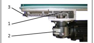
Do not over tension the drive chain. Proper tension should allow 2 to 6 mm of chain movement on the side.
