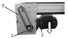
Do not over tension the drive chain. Proper tension should allow 2 to 6 mm of chain movement on the side.
