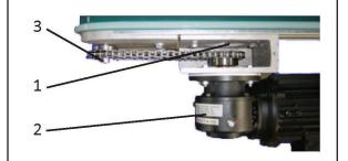
Do not over tension the drive chain. Proper tension should allow 2 to 6 mm of chain movement on the side.
