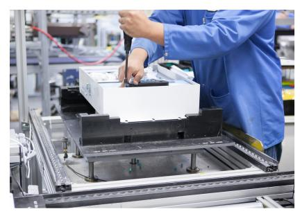
Manual screw-driving, is just one of the many processes that can be performed on a pallet conveyors. Here the pallet with product is also positioned and raised off the conveyor surface.
