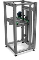
Figure 11: Vertical Transfer Unit
