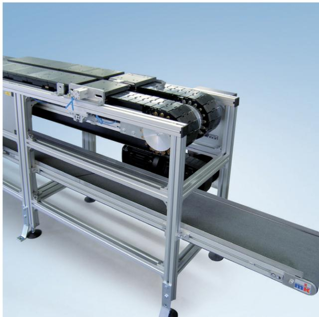
SPU 2040 interlink, dual-line with GUF-P 2000 belt conveyor as discharge belt for rejected parts.
