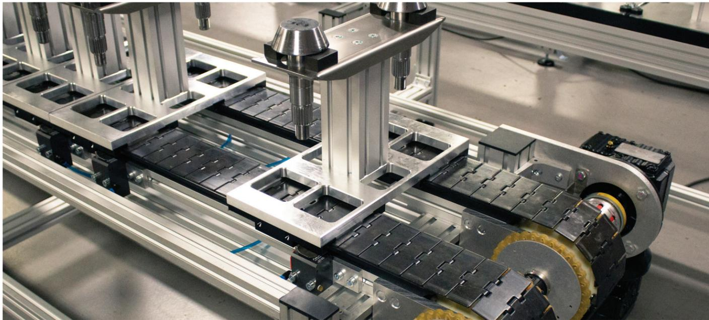
This SPU 2040 wide is carrying two parts on one pallet at once. The parts are queued before being offloaded.
