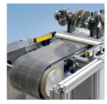
A special chain was used on this SPU 2040, along with roller strips for lateral positioning.
