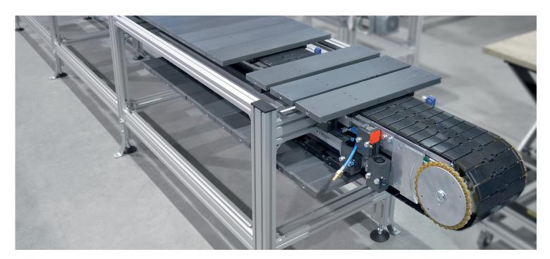
This is a SPU 2040, single lane (190 chain width) carrying a wide aluminum pallet, also featuring a pallet singulator.
