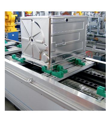
A SPU 2040 wide unit is used as an infeed conveyor for dishwasher
