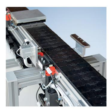
A locating device, with a pallet singulator, is shown on a 114 single
