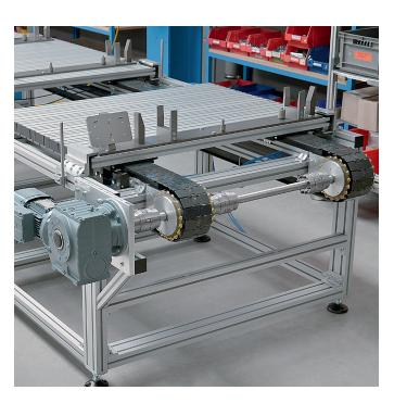
A SPU 2040, wide unit, with segmented profile based custom pallets.
