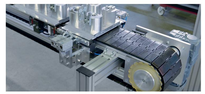
SPU 2040, single line with separating function and custom fixtures, for manual loading and automated removal.
