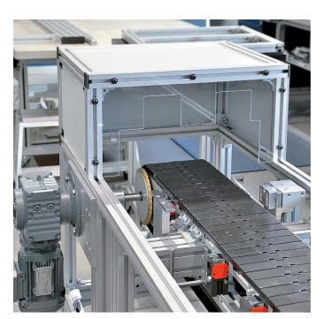
A protective guard with pendulum flap, mounted at the motor (discharge) end of a single lane unit.
