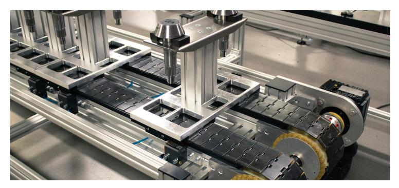
This SPU 2040 wide is carrying two parts on one pallet at once. The parts are queued before being offloaded.
