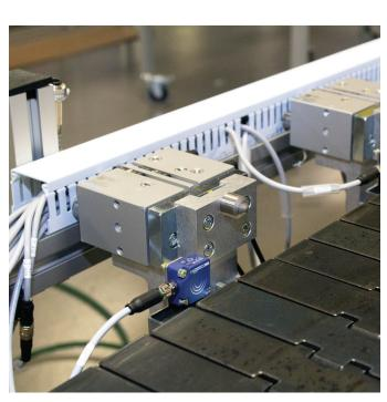
Locating pins are one half of the components that make up the locating device.
