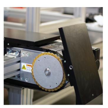
The Vulkolan® pressure pads ensure that the pallet transfers from the top to the return on the underside of the conveyor.
